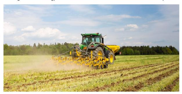
The STRIP-MASTER EN cultivator can be used for strip aeration up to a depth of 25 centimetres. We recommend aggregating the machine with **FERTI-BOX FB\_F or FERTI-CART FC, COMBO SYSTEM CS** for fertiliser application at two different layers. It is also possible to apply liquid fertilisers or manure and digestate.
