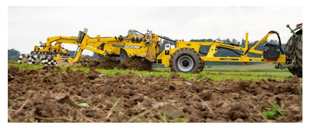
CADDY CD is equipped with wide transport wheels for safe transportation of the machine on roads. This equipment, together with the front weight, contributes to a good weight distribution and provides higher stability during transport.
